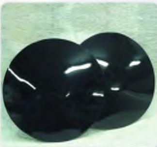
The disks are made in glass fibre or carbon fibre composites. They give your velomobile the additional aerodynamics and slightly better speed range as well as an aesthetic factor.
