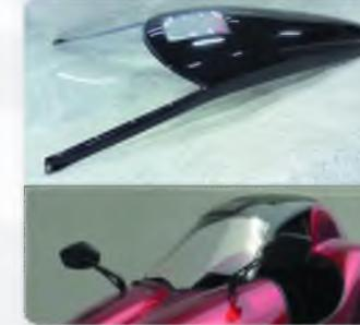
Made in glass fibre or carbon fibre composites. Designed to supplement Cab Bike Hawk in a perfect way.
